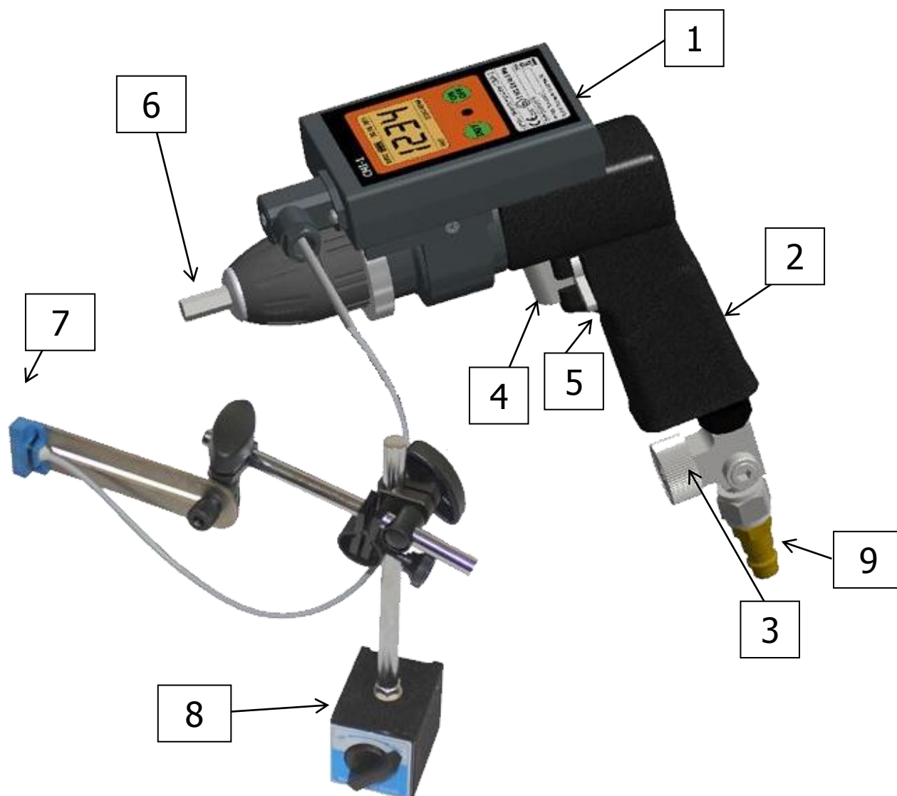
Fig.1 CMO-1 digital revolution meter - design
